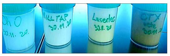
**Fig. 2.** Samples of pure coolant (a) not used in machining (Ch0) and used respectively from the tanks of the following machines: (b) four-axis milling machining center MILLTAP 700, (c) five-axis milling machine LASERTEC 65 SAUER, d) numerically controlled lathe CTX beta 1250 TC
